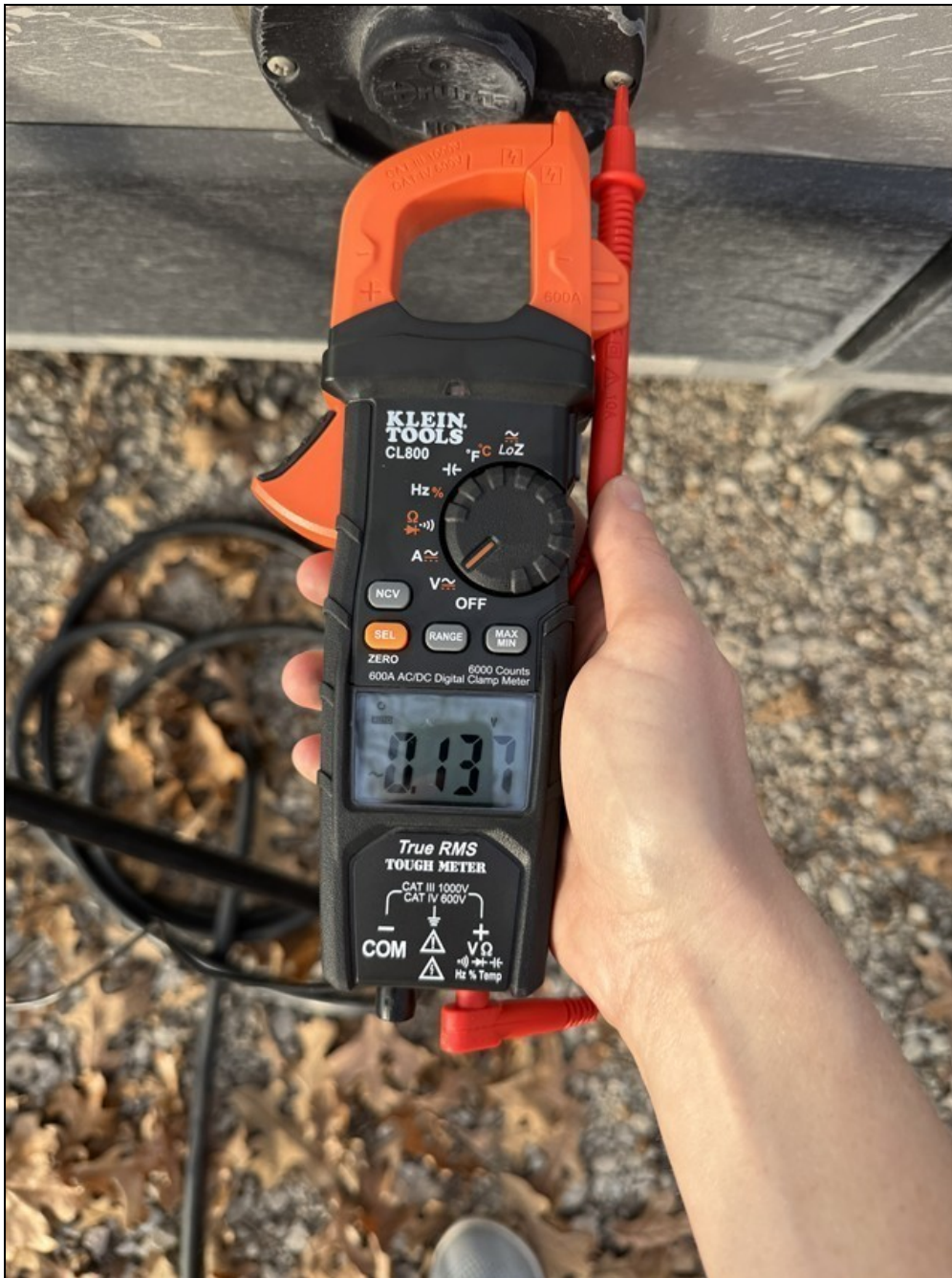
Hot Skin Test at Truma Water Heater Exterior Vent
